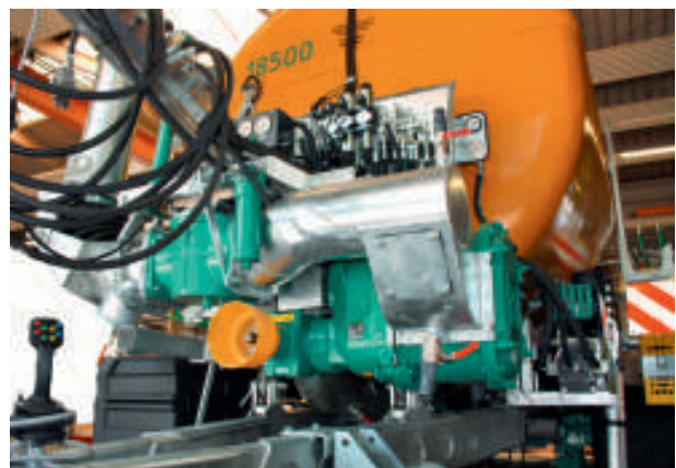
ECO-Pumpe Quereinbau links
